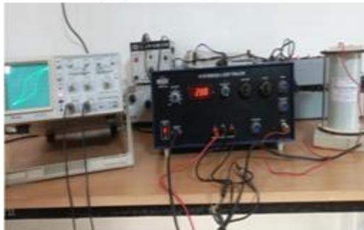
LCR Series and Parallel Resonance Circuit
