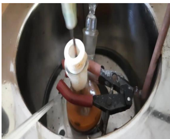
Fig.4: Experimental setup for epoxidation of fish oil.
