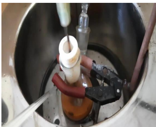
Fig.4: Experimental setup for epoxidation of fish oil.
