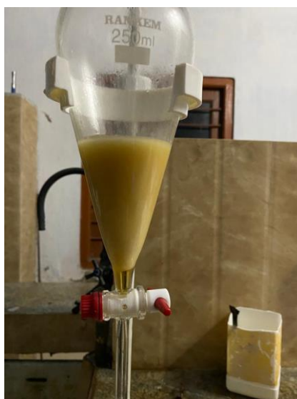
Fig.5: Synthesized epoxidized fish oil.
