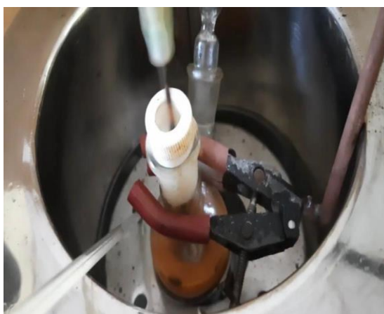
Fig.4: Experimental setup for epoxidation of fish oil.
