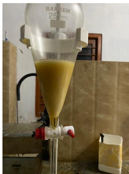
Fig.5: Synthesized epoxidized fish oil.
